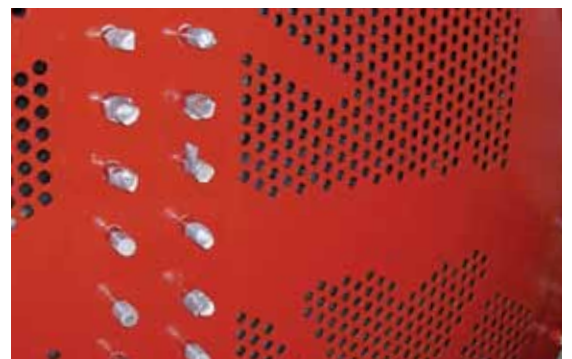
A tube sheet protected with Plastocor® 2000
